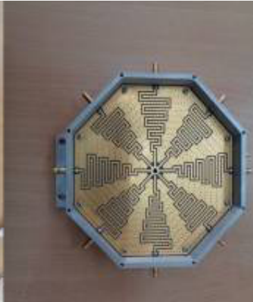
8- way power Combiner ( 8 kW) & splitter
