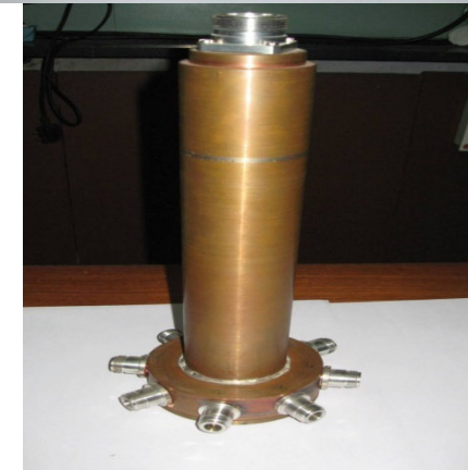
2.5 kW, 8 way Combiner
