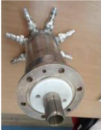
8- way power Combiner ( 8 kW) & splitter
